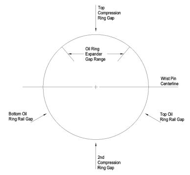
to prevent rotation of the oil rail support and the protruding dimple should be installed facing the bottom of the piston. This dimple should be postioned directly in line with the piston pin. Keep the oil rail support gap 90° from the piston pin bore
